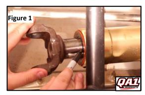
important to reference this point when making chassis adjustments, such as wheelbase or vehicle ride height, in order to verify the driveshaft does not bottom out in the transmission as the suspension moves through its full range of travel. If the driveshaft ever fully bottoms out on the transmission, it will damage the transmission or the driveshaft.
