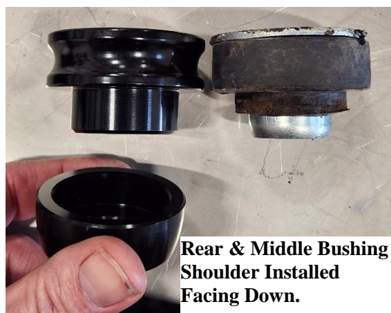
Front Bushing Position Shoulder UP.
