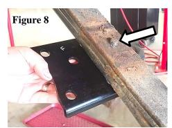
6) Install the larger plate to the bottom side of the leaf springs with the large hole in the plate towards the front of the truck and locating on the leaf spring centering pin. Secure the mounts re-using the factory U-bolts. (Figure 8) Evenly torque all U-bolt nuts to 74 lb. ft.
