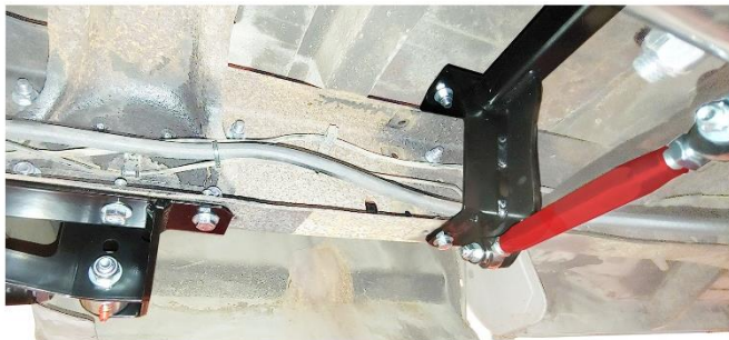
Stabilizer rod mounts directly to the torque arm crossmember Figure 29
