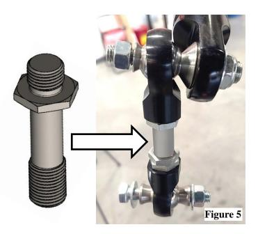
19. Check the clearance of the rod end and inner tie rod at full droop. Full droop is where these items will be closest to each other. Additional clearance can be gained by sliding the sway bar frame mount forward in its slotted holes.
