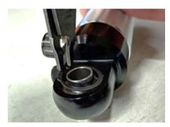
Using c-clip pliers, remove one c-clip and press the 1" wide bearing out of the shock eyelet. Install the 1.25" bearing included with the lower control arms and reinstall the c-clip. Push the c-clip into the shock eyelet to ensure it is seated.
