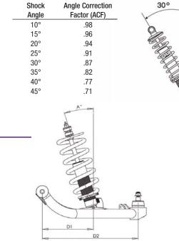
If your spring is mounted at an angle you will need to consider that in your spring calculations. Measure the angle (A) of your spring from vertical in degrees. Use the table above to determine your Angle Correction Factor (ACF). Now divide the Spring Force (Sf) from the earlier calculation by the Angle Correction Factor (ACF) to get the Adjusted Spring Force (ASf).
