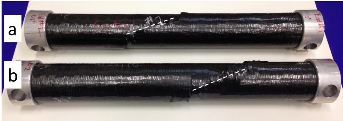
**Figure 5.** Failed full scale shafts a) unmodified control b) 48 wt% calcite-modified epoxy
