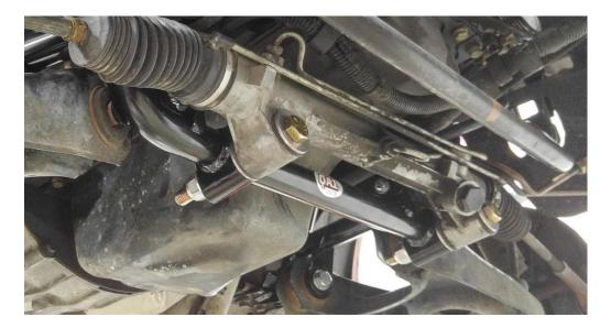
8. Tighten rack mounts using 15/16" socket/wrench until bushing diameter expands to same as washer.
