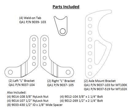
Warning: This kit does not contain all necessary components to convert from a leaf spring suspension to a link suspension. This kit contains shock mounts only.
