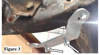
Before fully installing the bracket to the frame, install two 3/8" x 1" bolts into the center holes of the bracket facing down. (Figure 3)
