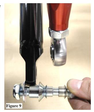
7. Attach sway bar to adjuster link using specialty high misalignment stud with ½" washer and nylock nut on the sway bar side. Attach link side using high misalignment spacer and a 3/8" nylock nut. Torque connection to 31 lb. (Figure 9)
