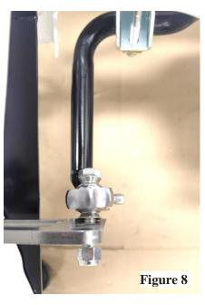
6. Attach one end of the assembled sleeve to the frame mount using two high misalignment spacers installed into the rod end. Fasten to frame mount using 3/8" x 2.5" bolts, with washer on the nylock nut side of the mount. The sway bar link will mount to the rear of the mount in the third hole from the top as a starting point. Torque to 31 lb. ft. (Figure 8)
